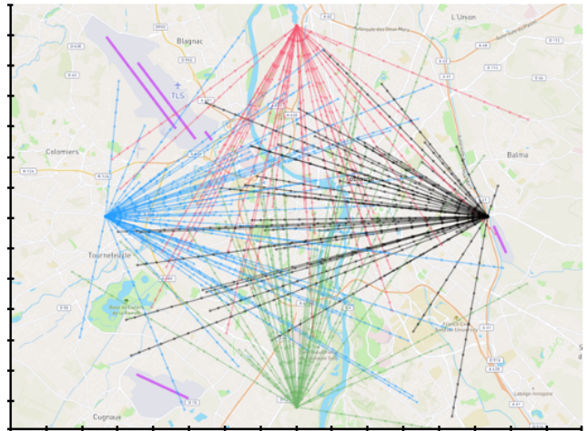
Fig. 1 Flight trajectories shown from 4 vertiports in a 16 \text{ km} \times 14 \text{ km} region, with axis ticks along the border denoting 1 km sector boundaries.
